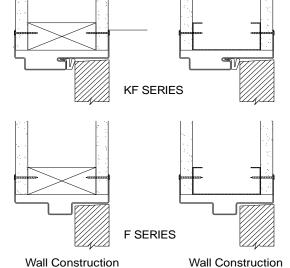
Wood Studs & Drywall Recommended Fasteners: 1-1/4" (min.) Drywall screws Coarse thread 6d common nails
