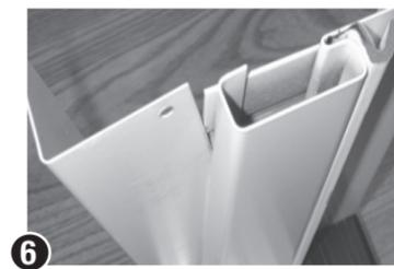
**6** On the other side of door, slide the jamb closure trims into the jambs, starting from bottom.
